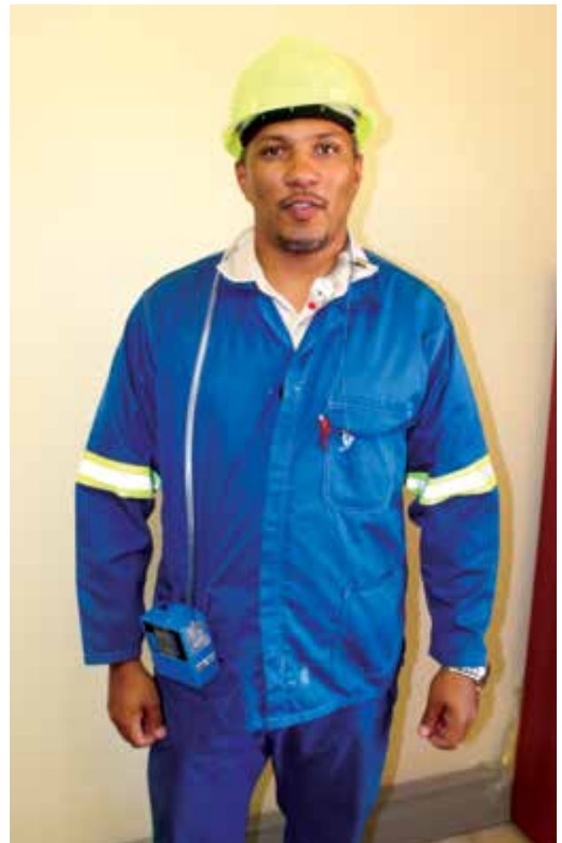
Correct use of personal dust sampler
