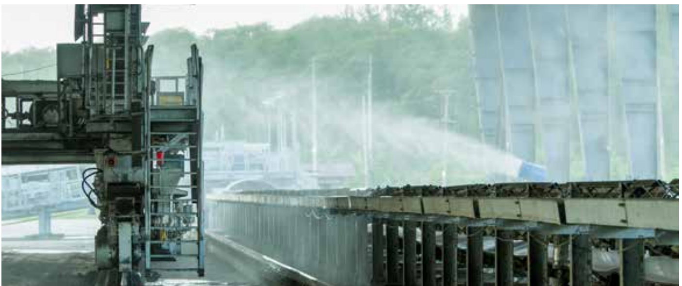
Watering down dust during ore transport on conveyor belt
