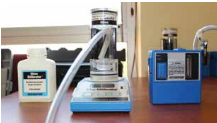
Personal dust sampling equipment including calibrator
